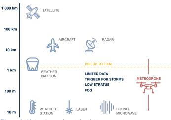
Figure 1: Meteodrone closes the data gap.
