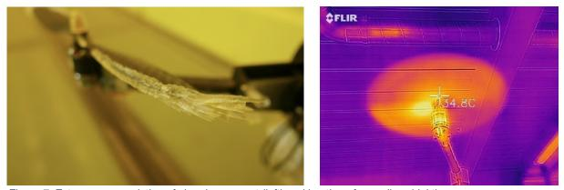
Figure 7: Extreme accumulation of clear ice amount (left) and heating of propellers (right).
