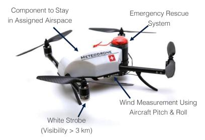
Each UAV is equipped with a ground station that enables a redundant telemetry link to the drone. All flight-relevant parameters are shown in realtime on a display attached to the ground station ensuring a direct monitoring of the flight. Hence, the pilot is able to keep track of the UAV at all times:
